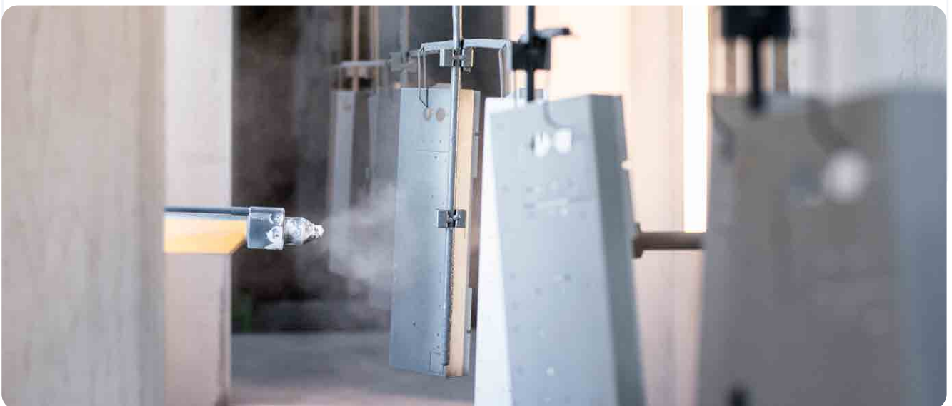
Thorlux powder coating facility utilising recycled powder
